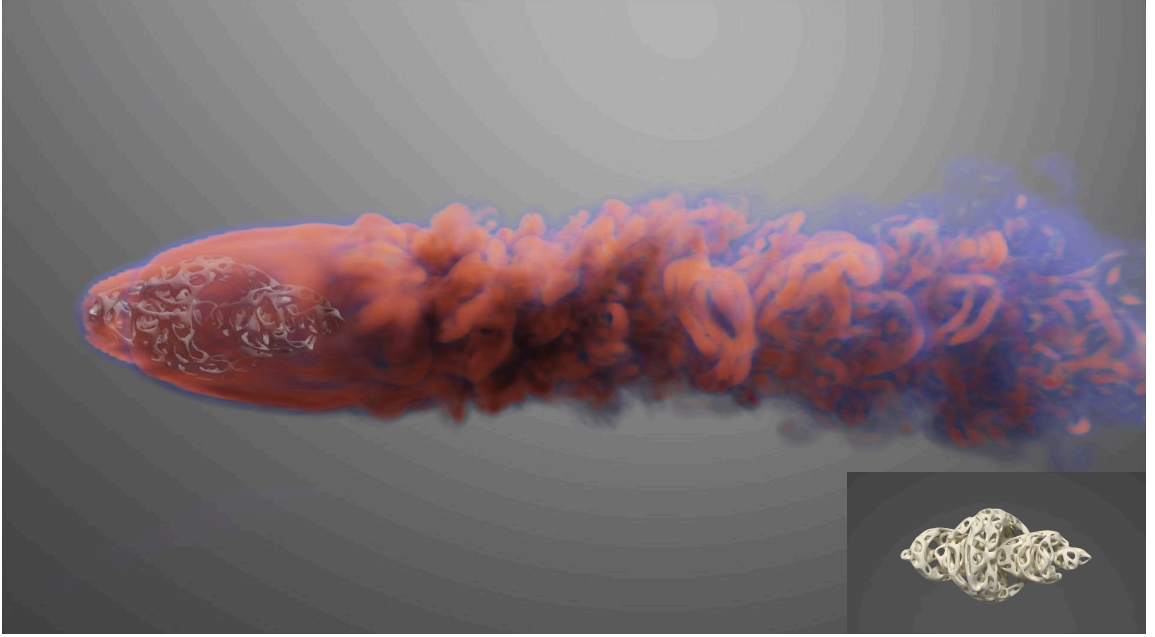
Fig. 17. Real-time 3D smoke simulation through a porous inlet with intricate microgeometry (128k triangle faces) on a 256 \times 128 \times 128 grid.
